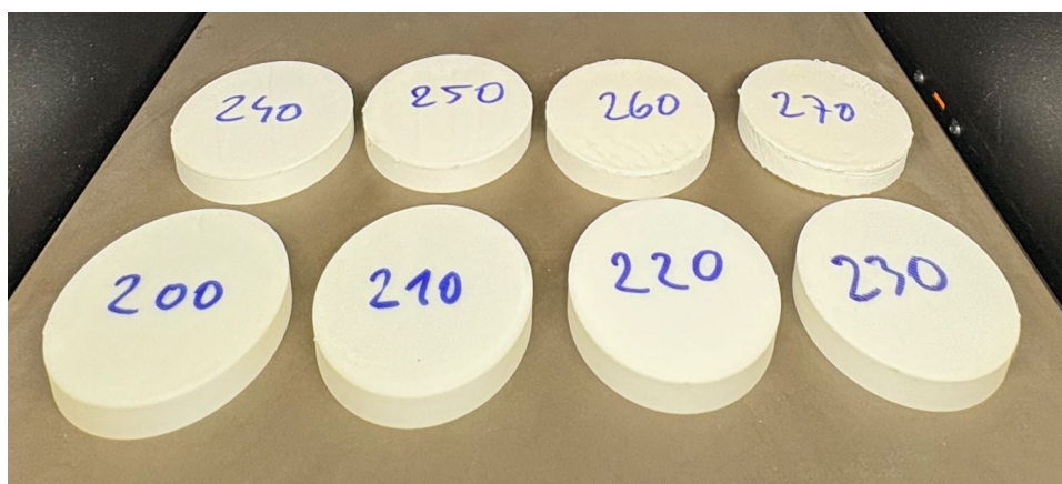
Fig. 1 Samples of the 200–270 °C temperature series, multiplier 1.00. Higher temperature gives a thicker wall and rougher surface.
